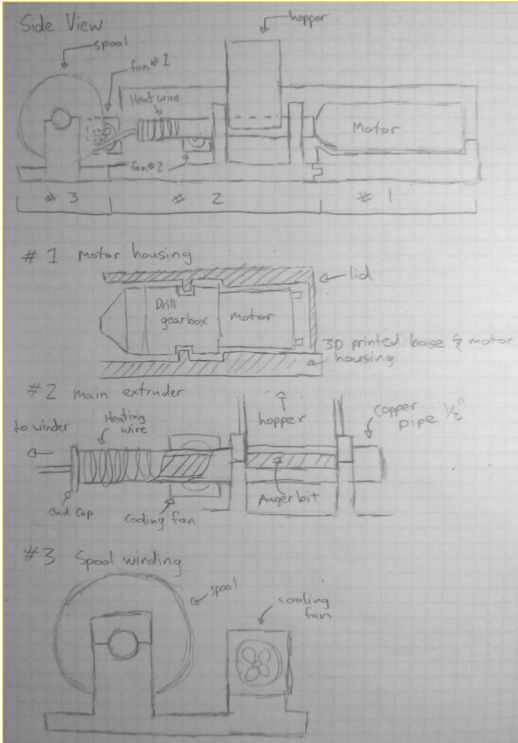
FIGURE 4- DESIGN SKETCHES OF THE PLASTIC EXTRUDER.
